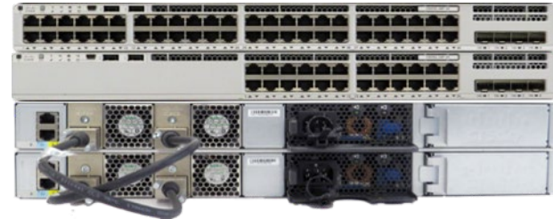
9200L Fixed Uplinks & Fans
